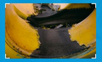
The vaporization surfaces of the injection nozzles are minimized and the odour substance can no longer be fully vaporized. Over time, the injection nozzles lose their function and – in extreme cases – can break off under the influence of the media flow and vibrations.
